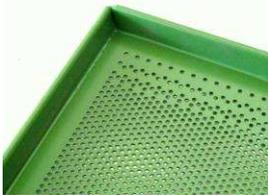
The perforation standard is obtained with a 2 mm diameter and 3.5 mm pitch. According to us, such dimensions achieve an optimal cooking and anti-adhesive ratio. Along the edges a band left full confers rigidity and consistency to tray.
