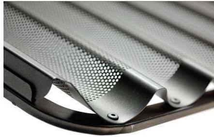
**CTIO\_T Corrugated perforated aluminium baking trays with stainless steel frame. 10/10 thickness. Natural, silicone or Teflon®-treated.**
